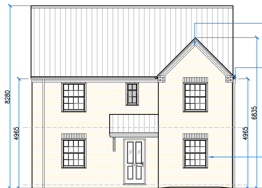
Proposed Front (South-East) Elevation PLOT 3 Scale 1:100
